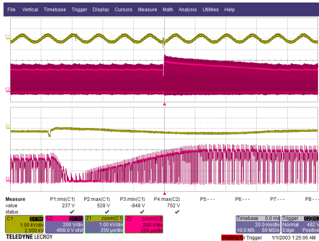
Figure 139 – DM Surge. V_{DS(MAX)} = 702 \text{ V}
