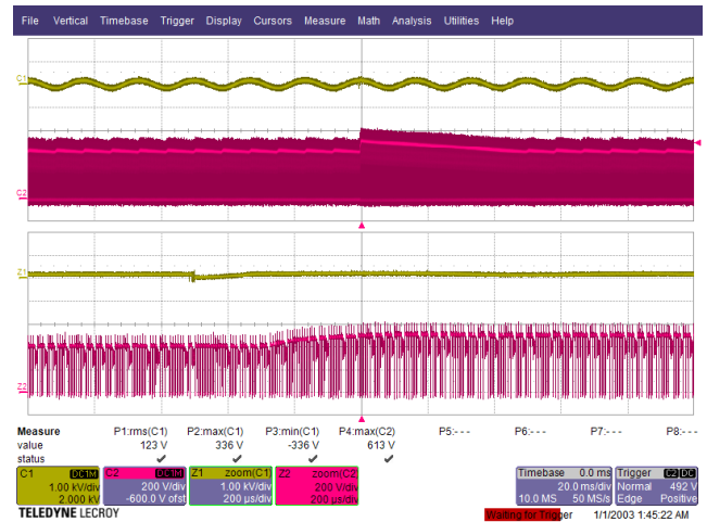
Figure 140 – CM Surge. V_{DS(MAX)} = 613 \text{ V}
