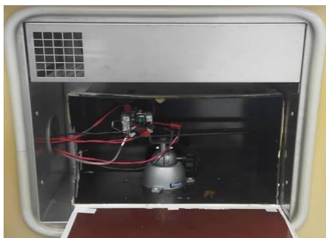
Figure 127 – Thermal Performance Set-up Using Thermal Chamber.
