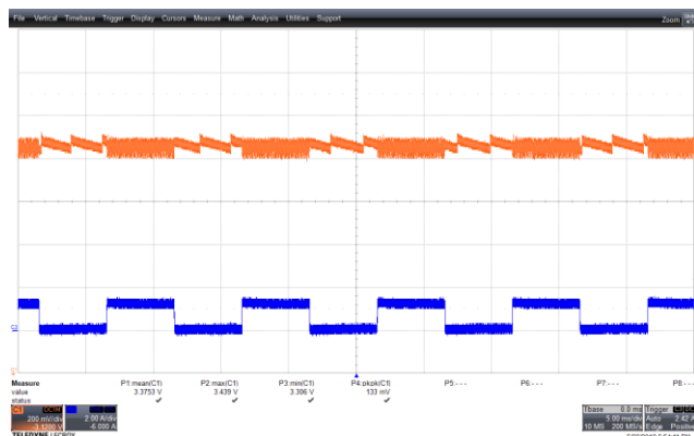
Figure 63 – Transient Response. 90 VAC, 3.3 V, 0 – 1.25 A Load Step. V_{MIN} : 3.306 V, V_{MAX} : 3.439 V. Upper: V_{OUT} , 0.2 V / div., 5 ms / div. Lower: I_{LOAD} , 2 A / div.
