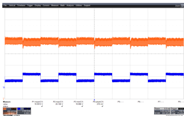
Figure 97 – Transient Response. 90 VAC, 20 V, 1.25 – 2.5 A Load Step. V_{MIN} : 19.886 V, V_{MAX} : 20.106 V. Upper: V_{OUT} , 0.2 V / div., 5 ms / div. Lower: I_{LOAD} , 2 A / div.
