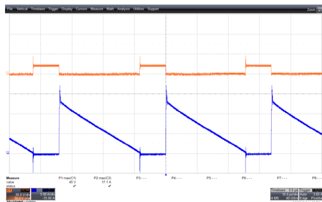
Figure 115 – SR FET Voltage Waveforms. 90 VAC, 5 V, 5 A Load, (45 V MAX ). Upper: SR_V DRAIN , 50 V / div., 10 µs / div. Lower: SR_I DRAIN , 5 A / div.
