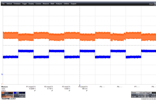
Figure 85 – Transient Response. 90 VAC, 9 V, 3.75 – 5 A Load Step. V_{MIN} : 8.92 V, V_{MAX} : 9.119 V. Upper: V_{OUT} , 0.2 V / div., 5 ms / div. Lower: I_{LOAD} , 2 A / div.
