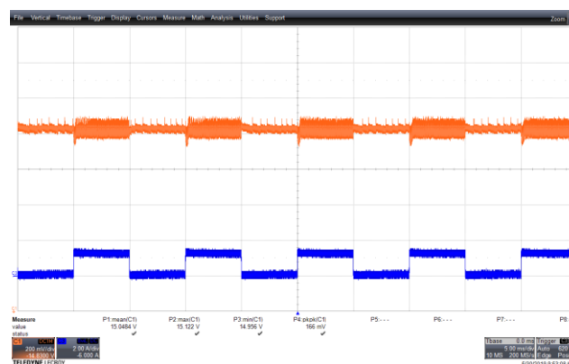
Figure 88 – Transient Response. 265 VAC, 15 V, 0 – 1.25 A Load Step. V_{\text{MIN}} : 14.956 V, V_{\text{MAX}} : 15.122 V. Upper: V_{\text{OUT}} , 0.2 V / div., 5 ms / div. Lower: I_{\text{LOAD}} , 2 A / div.
