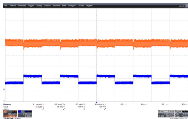
Figure 89 – Transient Response. 90 VAC, 15 V, 1.25 – 2.5 A Load Step. V_{\text{MIN}} : 14.916 V, V_{\text{MAX}} : 15.116 V. Upper: V_{\text{OUT}} , 0.2 V / div., 5 ms / div. Lower: I_{\text{LOAD}} , 2 A / div.
