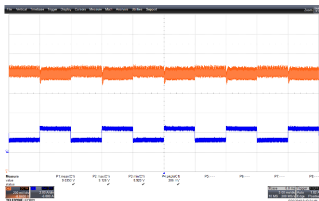
Figure 81 – Transient Response. 90 VAC, 9 V, 1.25 – 2.5 A Load Step. V_{MIN} : 8.92 V, V_{MAX} : 9.126 V. Upper: V_{OUT} , 0.2 V / div., 5 ms / div. Lower: I_{LOAD} , 2 A / div.
