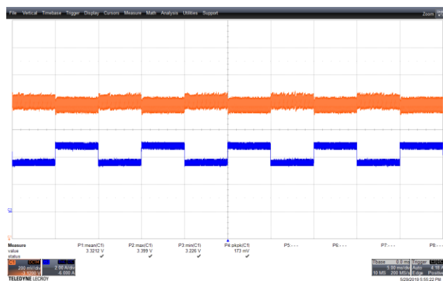
Figure 69 – Transient Response. 90 VAC, 3.3 V, 3.75 – 5 A Load Step. V_{MIN} : 3.226 V, V_{MAX} : 3.399 V. Upper: V_{OUT} , 0.2 V / div., 5 ms / div. Lower: I_{LOAD} , 2 A / div.
