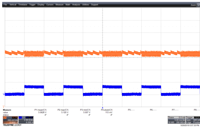
Figure 71 – Transient Response. 90 VAC, 5 V, 0 – 1.25 A Load Step. V_{MIN} : 5.007 V, V_{MAX} : 5.12 V. Upper: V_{OUT} , 0.2 V / div., 5 ms / div. Lower: I_{LOAD} , 2 A / div.
