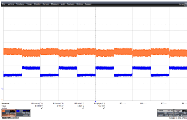
Figure 75 – Transient Response. 90 VAC, 5 V, 2.5 – 3.75 A Load Step. V_{MIN} : 4.934 V, V_{MAX} : 5.106 V. Upper: V_{OUT} , 0.2 V / div., 5 ms / div. Lower: I_{LOAD} , 2 A / div.
