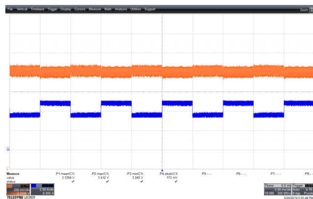
Figure 70 – Transient Response. 265 VAC, 3.3 V, 3.75 – 5 A Load Step. V_{MIN} : 3.240 V, V_{MAX} : 3.412 V. Upper: V_{OUT} , 0.2 V / div., 5 ms / div. Lower: I_{LOAD} , 2 A / div.
