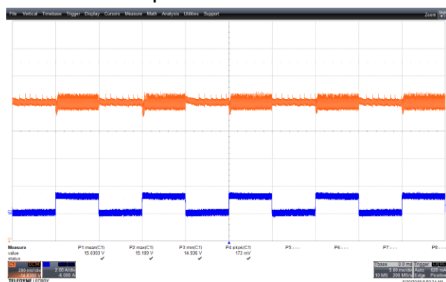
Figure 87 – Transient Response. 90 VAC, 15 V, 0 – 1.25 A Load Step. V_{\text{MIN}} : 14.936 V, V_{\text{MAX}} : 15.109 V. Upper: V_{\text{OUT}} , 0.2 V / div., 5 ms / div. Lower: I_{\text{LOAD}} , 2 A / div.
