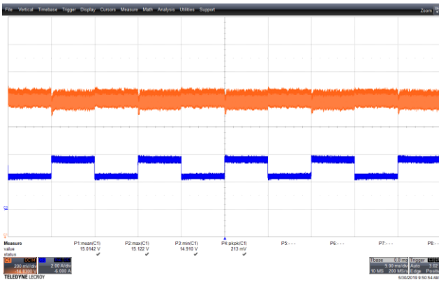
Figure 91 – Transient Response. 90 VAC, 15 V, 2.5 – 3.75 A Load Step. V_{MIN} : 14.91 V, V_{MAX} : 15.122 V. Upper: V_{OUT} , 0.2 V / div., 5 ms / div. Lower: I_{LOAD} , 2 A / div.
