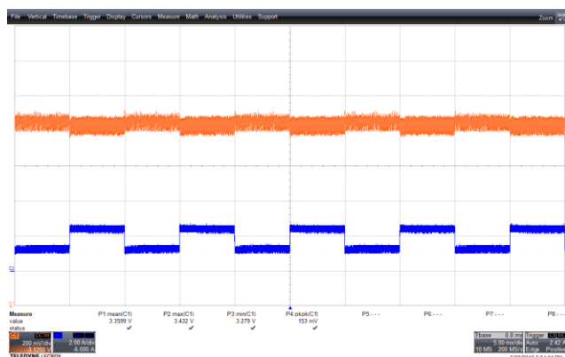
Figure 65 – Transient Response. 90 VAC, 3.3 V, 1.25 – 2.5 A Load Step. V_{MIN} : 3.279 V, V_{MAX} : 3.432 V. Upper: V_{OUT} , 0.2 V / div., 5 ms / div. Lower: I_{LOAD} , 2 A / div.
