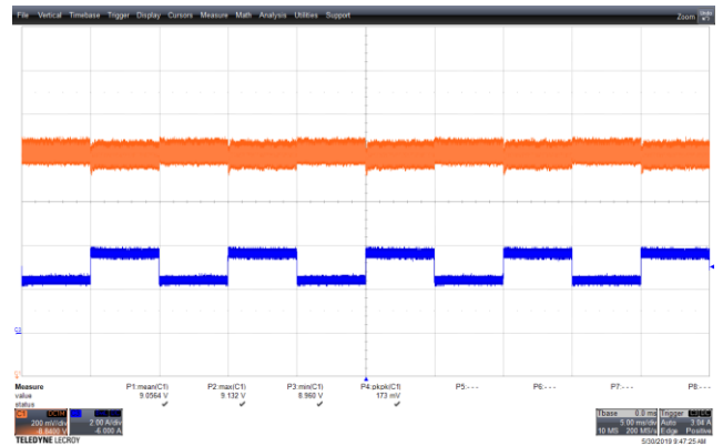
Figure 84 – Transient Response. 265 VAC, 9 V, 2.5 – 3.75 A Load Step. V_{MIN} : 8.96 V, V_{MAX} : 9.132 V. Upper: V_{OUT} , 0.2 V / div., 5 ms / div. Lower: I_{LOAD} , 2 A / div.
