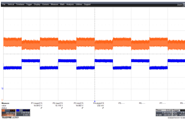
Figure 93 – Transient Response. 90 VAC, 15 V, 3.75 – 5 A Load Step. V_{MIN} : 14.883 V, V_{MAX} : 15.116 V. Upper: V_{OUT} , 0.2 V / div., 5 ms / div. Lower: I_{LOAD} , 2 A / div.
