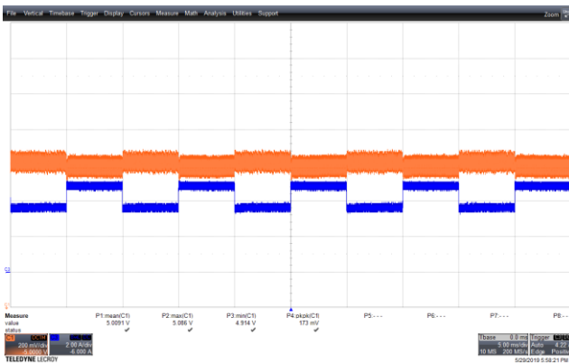
Figure 77 – Transient Response. 90 VAC, 5 V, 3.75 - 5 A Load Step. V_{MIN} : 4.914 V, V_{MAX} : 5.086 V. Upper: V_{OUT} , 0.2 V / div., 5 ms / div. Lower: I_{LOAD} , 2 A / div.
