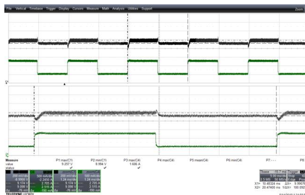
Figure 56 – Transient Response. 265 VAC, 9.0 V, 0.75 – 1.5 A Load Step. V_{MIN} : 8.994 V, V_{MAX} : 9.257 V. Upper: V_{OUT} , 0.2 V / div., 53 ms / div. Lower: I_{LOAD} , 1 A / div. Zoom: 1.46 ms / div.
