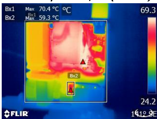
Figure 39 – Top Side Thermal Image. Ambient: 24.6 °C. Bx1: Transformer Winding = 70.4 °C. Bx2: Thermistor RT1 = 59.3 °C.
