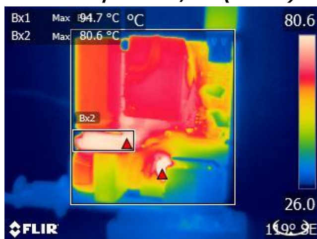
Figure 37 – Top Side Thermal Image. Ambient: 25.6 °C. Bx1: Thermistor RT1 = 94.7 °C. Bx2: Bridge Rectifier BR1 = 80.6 °C
