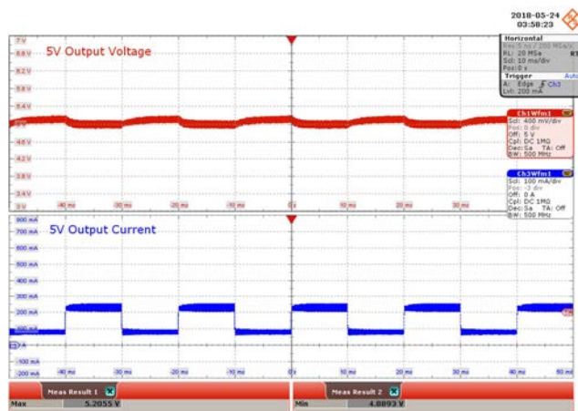
Figure 55 – 85 VAC Input. Upper: 5 V V_{OUT} , 400 mV / div., 10 ms / div. Lower: 5 V I_{OUT} , 100 mA / div. V_{MAX} : 5.2055 V. V_{MIN} : 4.8893 V.
