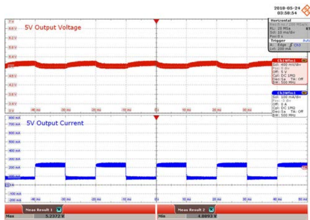
Figure 55 – 85 VAC Input. Upper: 5 V V_{OUT} , 400 mV / div., 10 ms / div. Lower: 5 V I_{OUT} , 100 mA / div. V_{MAX} : 5.2055 V. V_{MIN} : 4.8893 V.
