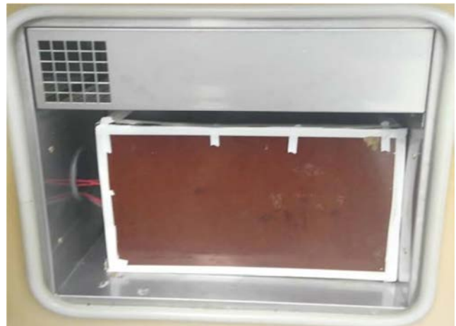
Figure 74 – Thermal Performance Set-up Using Thermal Chamber.
