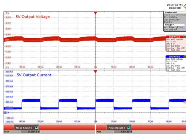
Figure 56 – 115 VAC Input. Upper: 5 V V_{OUT} , 400 mV / div., 10 ms / div. Lower: 5 V I_{OUT} , 100 mA / div. V_{MAX} : 5.2055 V. V_{MIN} : 4.8893 V.
