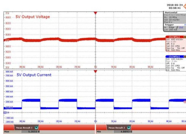
Figure 56 – 115 VAC Input. Upper: 5 V V_{OUT} , 400 mV / div., 10 ms / div. Lower: 5 V I_{OUT} , 100 mA / div. V_{MAX} : 5.2055 V. V_{MIN} : 4.8893 V.
