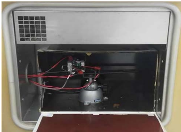
Figure 74 – Thermal Performance Set-up Using Thermal Chamber.
