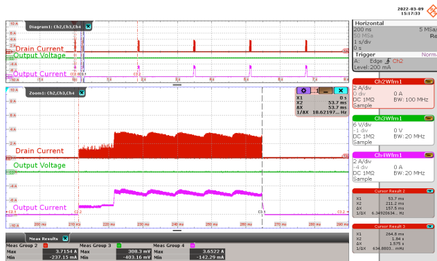
Figure 34 – Drain Current and Output Waveforms. 85 VAC Input.
