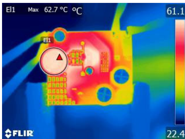
Figure 12 – Buck Choke (EI1), 62.7 °C. 85 VAC, 800 mA Output.
