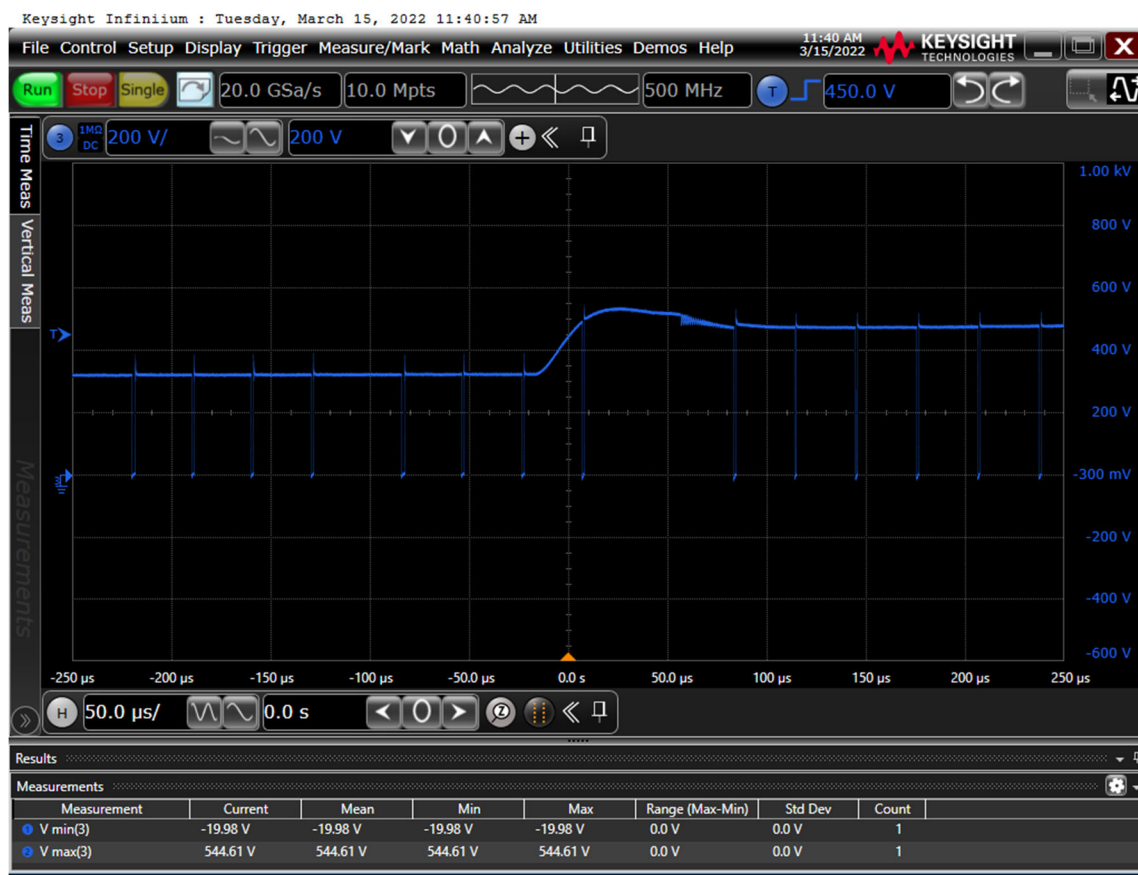
Figure 97 – Drain Voltage, 230 VAC, Full Load.
