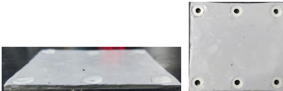
Figure 212 – Assembled Aluminum Sheet, Thermal Pad, and spacer.
