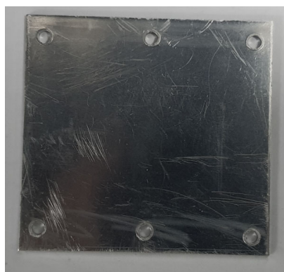
Figure 210 – Cut Aluminum Sheet with Hole.
