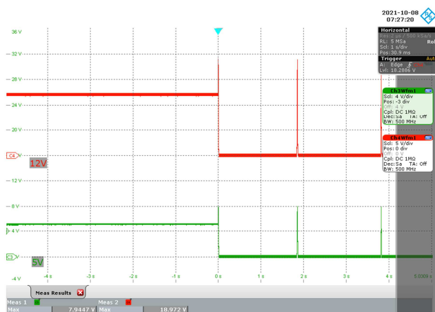
Figure 144 – 265 VAC 60 Hz. Full Load.
