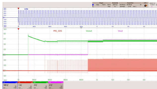
Figure 54 – Output Voltage at Start-up. 265 VAC, 5 V, 3 A Load.
