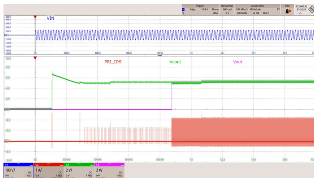
Figure 53 – Output Voltage at Start-up. 90 VAC, 5 V, 3 A Load.
