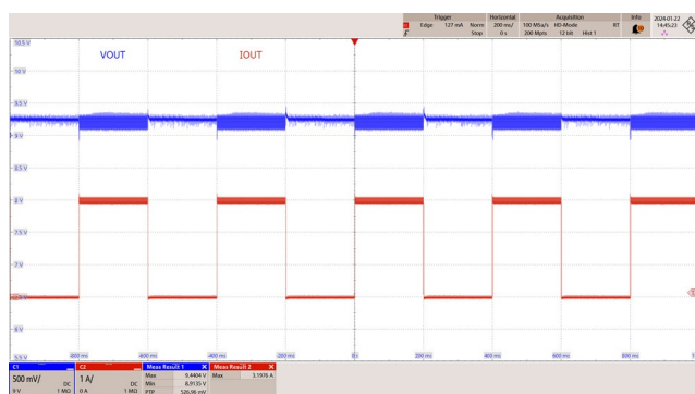
Figure 63 – Transient Response. 90 VAC, 9 V, 0% – 100% Load Step. V_{MIN} : 8.914 V, V_{MAX} : 9.44 V. C1: V_{OUT} , 500 mV / div. C2: I_{OUT} , 1 A / div. Time: 200 ms / div.
