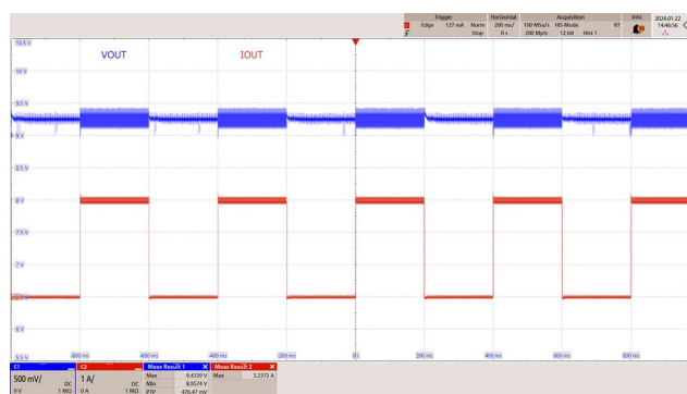
Figure 64 – Transient Response. 265 VAC, 9 V, 0% – 100% Load Step. V_{MIN} : 8.957 V, V_{MAX} : 9.434V. C1: V_{OUT} , 500 mV / div. C2: I_{OUT} , 1 A / div. Time: 200 ms / div.
