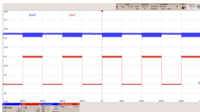
Figure 61 – Transient Response. 90 VAC, 5 V, 0% – 100% Load Step. V_{MIN} : 4.929 V, V_{MAX} : 5.324 V. C1: V_{OUT} , 500 mV / div. C2: I_{OUT} , 1 A / div. Time: 200 ms / div.
