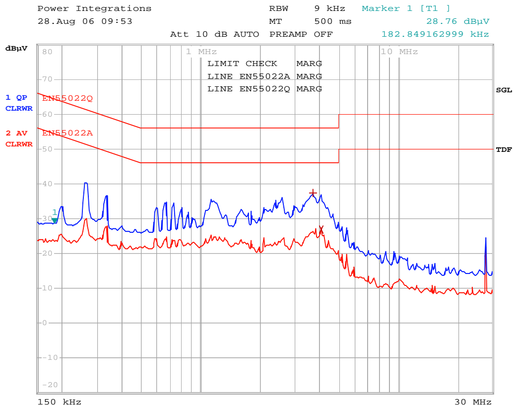
Figure 27 – Conducted EMI, Maximum Steady State Load, 230 VAC, 60 Hz, and EN55022 B Limits.
