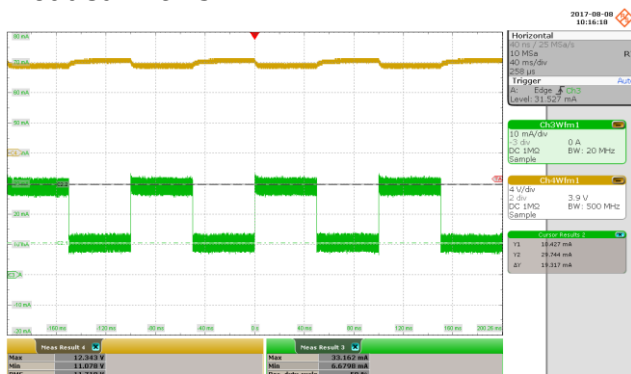
Figure 27 – 85 VAC, 0-100% Load Step. V_{MAX} : 12.343 V. V_{MIN} : 11.078 V. Upper: V_{OUT} , 4 V / div. Lower: I_{LOAD} , 10 mA / div., 40 ms / div.
