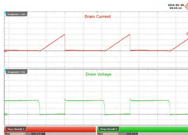
Figure 70 – 90 VAC, 48 V LED Load. Upper: I_{DRAIN} , 100 mA / div. Lower: V_{DRAIN} , 50 V / div., 5 μs / div.
