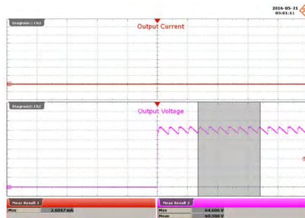
Figure 94 – 300 VAC, Open Load. Open Load Start-up. Upper: I_{OUT} , 40 mA / div. Lower: V_{OUT} , 10 V / div., 4 s / div.
