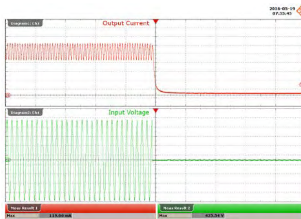
Figure 68 – 230 VAC, 48 V LED, Output Fall. Upper: I_{OUT} , 40 mA / div. Lower: V_{IN} , 100 V / div., 100 ms / div.
