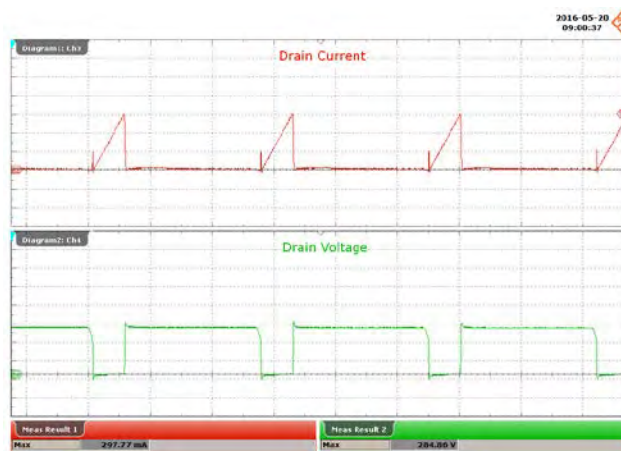
Figure 74 – 230 VAC, 48 V LED Load. Upper: I_{DRAIN} , 100 mA / div. Lower: V_{DRAIN} , 100 V / div., 5 μs / div.
