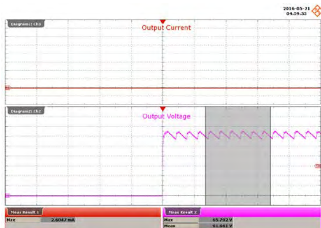
Figure 93 – 230 VAC, Open Load. Open Load Start-up. Upper: I_{OUT} , 40 mA / div. Lower: V_{OUT} , 10 V / div., 4 s / div.
