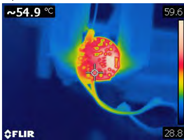
Figure 17 – 90 VAC, 48 V LED Load. Spot 1: Flywheel Diode (D1): 54.9 °C.
