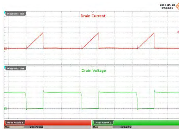
Figure 72 – 115 VAC, 48 V LED Load. Upper: I_{DRAIN} , 100 mA / div. Lower: V_{DRAIN} , 50 V / div., 5 μs / div.
