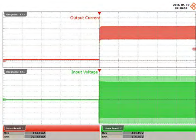
Figure 63 – 30 VAC, 48 V LED, Output Rise. Upper: I_{OUT} , 40 mA / div. Lower: V_{IN} , 100 V / div., 1 s / div.
