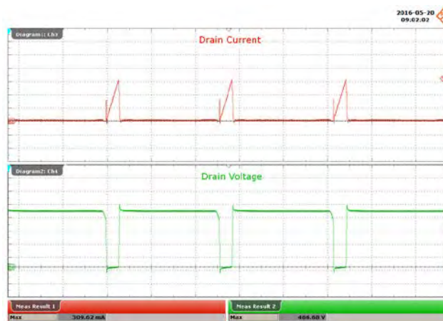
Figure 76 – 300 VAC, 48 V LED Load. Upper: I_{DRAIN} , 100 mA / div. Lower: V_{DRAIN} , 100 V / div., 5 μs / div.
