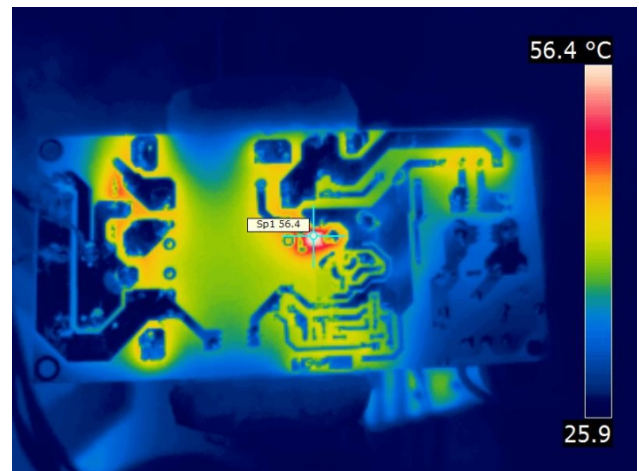
Figure 19 – Blocking Diode D4 (Sp1) Case Temperature.
