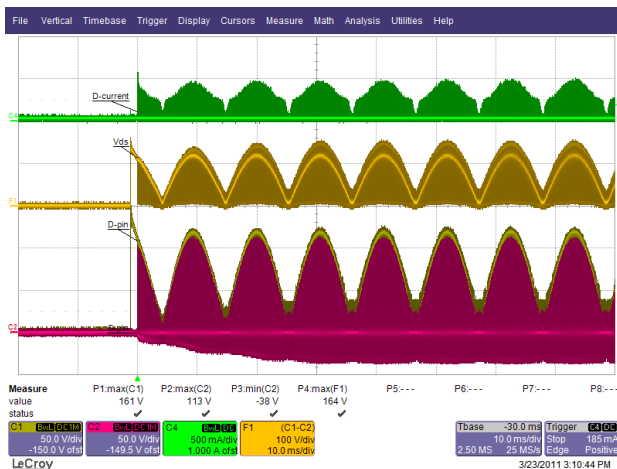
Figure 29 – 85 VAC / 47 Hz, 35 V LED String.
