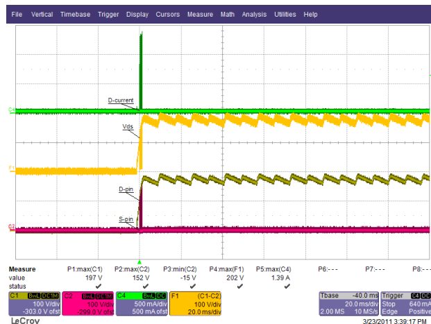
Figure 39 – 135 VAC / 63 Hz, Output Shorted.
