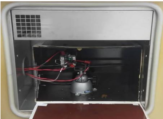
Figure 127 – Thermal Performance Set-up Using Thermal Chamber.
