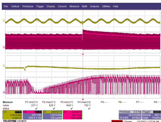
Figure 139 – DM Surge. V_{DS(MAX)} = 702 \text{ V}
