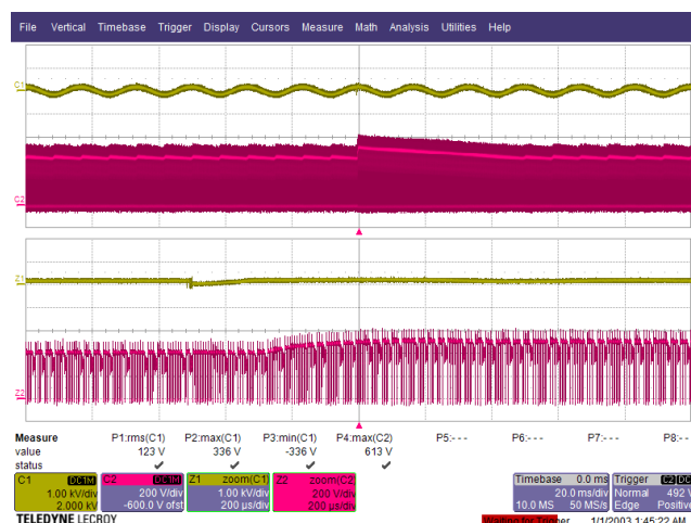
Figure 140 – CM Surge. V_{DS(MAX)} = 613 \text{ V}
