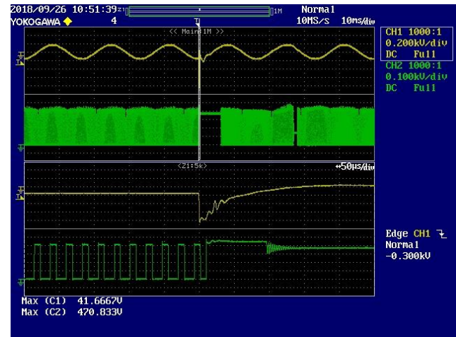
Figure 131 – (-)1 kV Differential Surge, 270° Phase Angle. Lower: V_{DRAIN} , 100 V / div., 10 ms / div. Peak V_{DRAIN} : 470.83 V.
