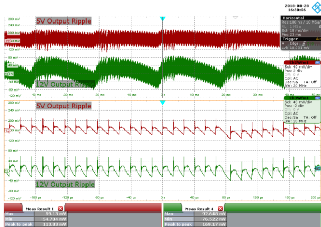
Figure 110 – 85 VAC 60 Hz, 100% Load. CH2: 5 V OUT , 40 mV / div., 10 ms / div. CH3: 12 V OUT , 40 mV / div., 10 ms / div. Zoom: 40 μs / div. 5 V Output Ripple = 113.83 mV. 12 V Output Ripple = 169.17 mV.
