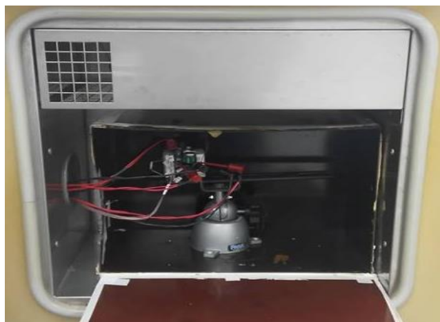
Figure 74 – Thermal Performance Set-up Using Thermal Chamber.
