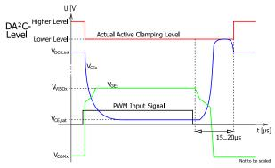
Figure 6. Dynamic Advanced Active Clamping (DA<sup>2</sup>C).
