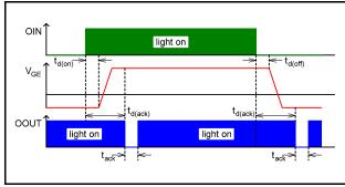
Figure 3. Driver Behavior and Status Feedback in Normal Operation
