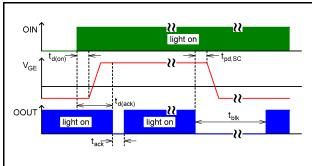
Figure 4. Driver Behavior and Status Feedback during Short-Circuit
