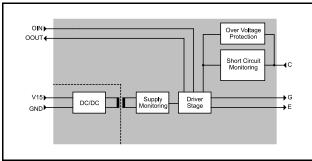
Figure 2. Functional Block Diagram.
