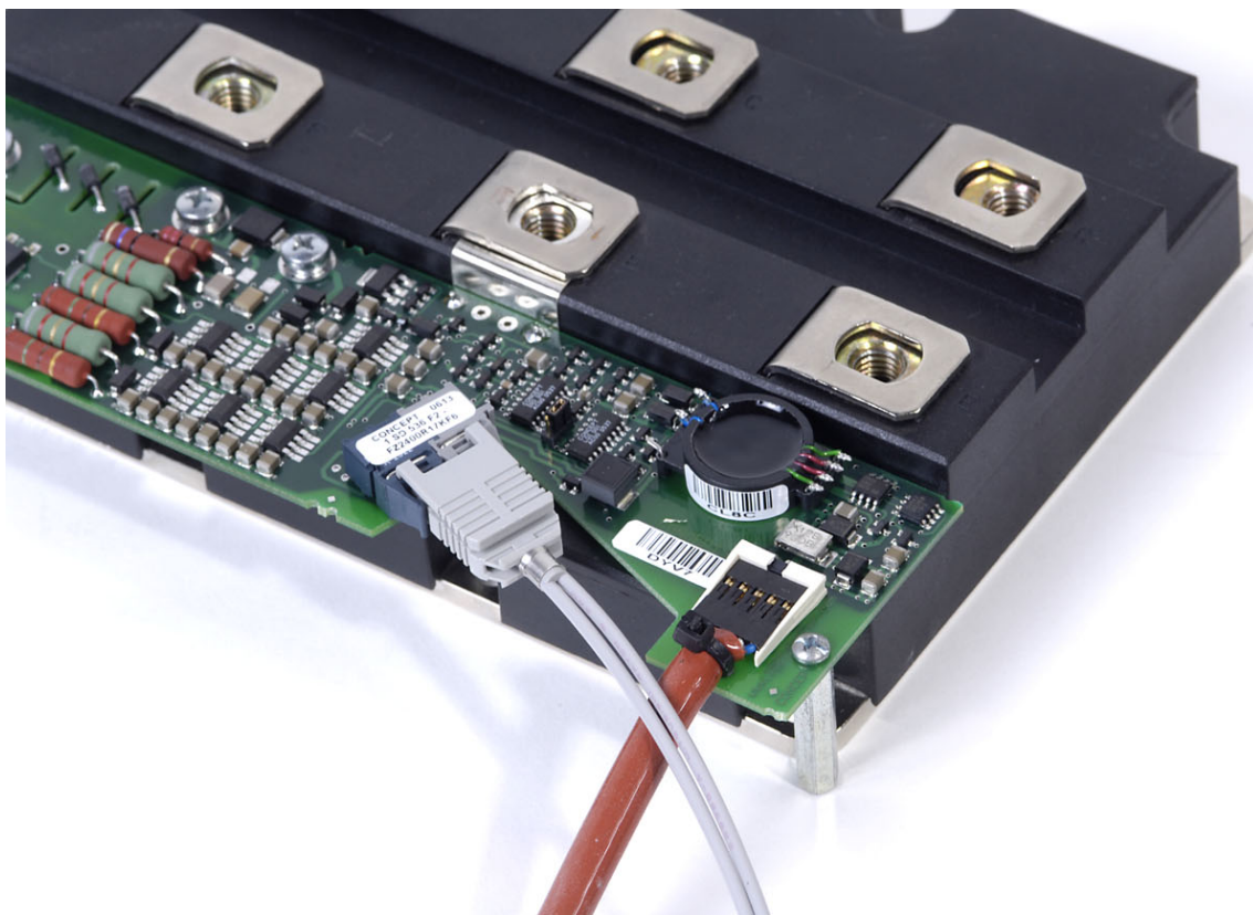
Fig. 16 Additional measures for fixing driver and power-supply cables as well as the relevant version of interlocking fiber-optic links
