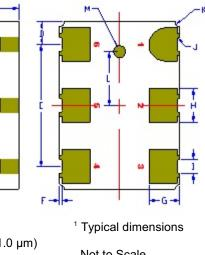
Contacts (pads): Gold 11.8 to 39.4 µinches (0.3 to 1.0 µm) over Nickel 50 to 350 µinches (1.27 to 8.89 µm)
