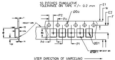
REEL DIMENSIONS 7.0 10.0 13.0 А inches mm 177.8 254.0 330.2 2.50 в inches 4.00 3.75 mm 63.5 101.6 95.3 Таре Width С mm 13.0 +0.5 / -0.2 8.4 +2.0 -0.0 D mm 8.4 8.4 8.0 +2.0 -0.0 +2.0 -0.0
