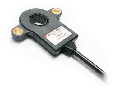
The PST-360 through / hollow shaft position sensors combines three critical design features; 1) through hole where the shaft passes through the sensor, 2) high accuracy absolute position feedback over up to 360°, and 3) a true non-contacting sensing element. Piher's design does not rely on gears or other rotating parts.
