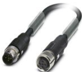
Sensor/actuator cable, 5-position, PUR halogen-free, black-gray RAL 7021, shielded, Plug straight M12 SPEEDCON, A - standard, on Socket straight M12 SPEEDCON, A - standard, cable length: 3 m
