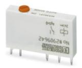
Plug-in miniature power relay, with power contact, 1 changeover contact, manual operation, 24 V DC input voltage
