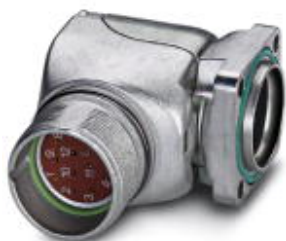
Device connector, front mounting, angled fixed, Screw locking, M23, number of positions: 12, type of contact: Socket, Crimp connection, Axial O-ring, 4x Ø 3.2, shielded: yes, flange dimensions: 26 mm x 26 mm
