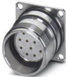
Device connector for rear wall, straight, Screw locking, M23, No. of pos.: 6+3, type of contact: Socket, Solder-in connection, Radial O-ring, 4x Ø 3.2, Panel thickness min.: 2.7 mm, Panel thickness max.: 3.5 mm
