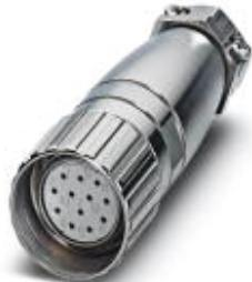
Cable connector, with Pg11 connection thread, straight, shielded: yes, Screw locking, M23, No. of pos.: 17, type of contact: Socket, Crimp connection, cable diameter range: 7.5 mm ... 9.5 mm
