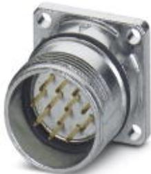
Device connector for front wall, straight, shielded: yes, Screw locking, M23, No. of pos.: 17, type of contact: Pin, Solder connection, Radial O-ring, 4x Ø 3.2
