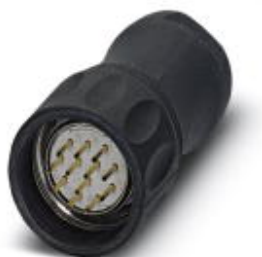
Cable connector, straight plastic-sheathed, shielded: yes, Screw locking, M23, No. of pos.: 16, type of contact: Pin, Solder connection
