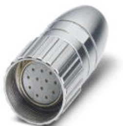
Cable connector, straight, shielded: yes, Screw locking, M23, No. of pos.: 12, type of contact: Socket, Solder connection
