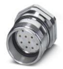
Device connector with Pg13.5 screw-in thread, straight, shielded: yes, Screw locking, M23, No. of pos.: 12, type of contact: Socket, Crimp connection, Axial O-ring, Central fixing, Panel thickness min.: 1 mm, Panel thickness max.: 4.5 mm
