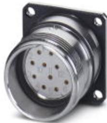
Device connector for rear wall, straight, Screw locking, M23, No. of pos.: 12, type of contact: Socket, Solder connection, Flat gasket, 4x M2.5
