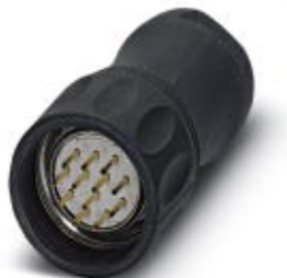
Cable connector, straight plastic-sheathed, shielded: yes, Screw locking, M23, No. of pos.: 12, type of contact: Pin, Crimp connection
