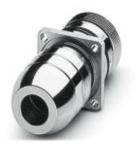
Feed-through of front wall, straight, shielded: yes, Screw locking, M23, No. of pos.: 8+1, type of contact: Socket, Solder connection, Flat gasket, 4x Ø 3.2, Panel thickness min.: 3 mm, Panel thickness max.: 7 mm, cable diameter range: 7.5 mm ... 9.5 mm
