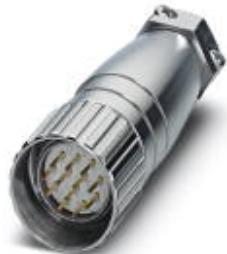
Cable connector, with Pg9 connection thread, straight, shielded: yes, Screw locking, M23, No. of pos.: 8+1, type of contact: Pin, Crimp connection, cable diameter range: 6.5 mm ... 7.5 mm
