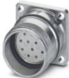
Device connector for front wall, straight, shielded: yes, Screw locking, M23, No. of pos.: 7, type of contact: Socket, Solder connection, Radial O-ring, 4x Ø 3.2
