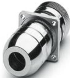
Feed-through of front wall, straight, shielded: yes, Screw locking, M23, No. of pos.: 6, type of contact: Socket, Crimp connection, Flat gasket, 4x Ø 3.2, Panel thickness min.: 3 mm, Panel thickness max.: 7 mm, cable diameter range: 9.5 mm ... 10.5 mm
