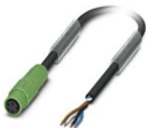
Sensor/actuator cable, 4-position, PUR halogen-free, black-gray RAL 7021, free cable end, on Socket straight M8, cable length: 1 m
