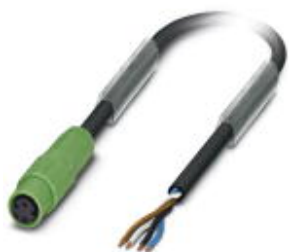
Sensor/actuator cable, 4-position, PUR halogen-free, black-gray RAL 7021, free cable end, on Socket straight M8, cable length: 0.5 m
