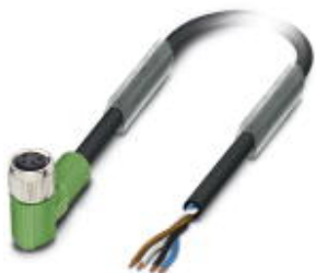
Sensor/actuator cable, 4-position, PUR/PVC, gray RAL 7001, free cable end, on Socket angled M8, cable length: 5 m
