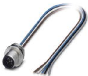
Sensor/Actuator flush-type plug, 5-pos., M12, A-coded, front/screw mounting with M16 thread, with 1.5 m TPE litz wire, 5 x 0.34 mm²
