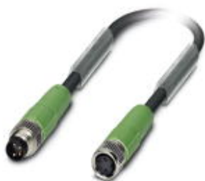
Sensor/actuator cable, 4-position, PUR halogen-free, black-gray RAL 7021, shielded, Plug straight M8, on Socket straight M8, cable length: 10 m
