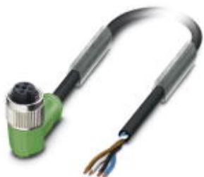
Sensor/actuator cable, 4-position, PUR/PVC, yellow, free cable end, on Socket angled M12, A-coded, cable length: 5 m
