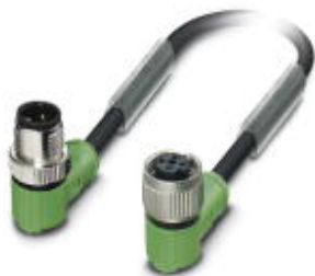
Sensor/actuator cable, 4-position, PUR halogen-free, black-gray RAL 7021, Plug angled M12 SPEEDCON, A-coded, on Socket angled M12 SPEEDCON, A-coded, cable length: 15 m
