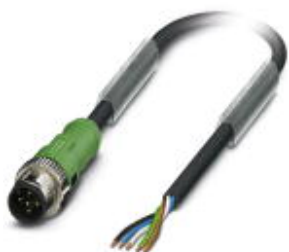
Sensor/actuator cable, 5-position, PUR, black-gray RAL 7021, Plug straight M12 SPEEDCON, A-coded, on free cable end, cable length: 2.7 m
