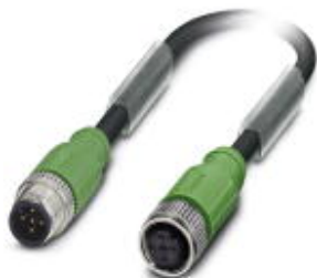
Sensor/actuator cable, 5-position, PUR halogen-free, black-gray RAL 7021, shielded, Plug straight M12, on Socket straight M12, cable length: 5 m
