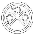
Pin assignment of M12 socket, 3-pos., S-coded, socket side view
