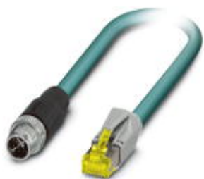
Network cable, Ethernet CAT5, 8-position, PUR, water blue RAL 5021, shielded, Plug straight M12 SPEEDCON / IP67, cable length: 7.5 m
