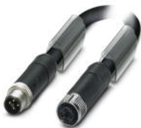
Power cable, 4-position, PUR halogen-free, black-gray RAL 7021, Plug straight M12, T-coded, on Socket straight M12, T-coded, cable length: 0.5 m
