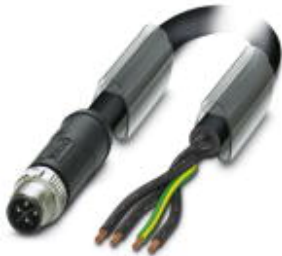
Sensor/actuator cable, 4-position, PUR halogen-free, black-gray RAL 7021, Plug straight M12 SPEEDCON, S-coded, on free cable end, cable length: 0.5 m, for AC current up to 12 A/630 V
